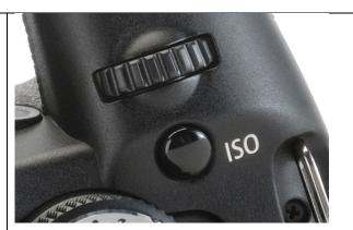
Digital cameras work like film, only the film is the sensor, which stores information in pixels on your memory card. It is the most costly piece of real estate on your camera. The ISO determines the level of sensitivity to light that this sensor reacts to, in the environment you expose it to. How that image sensor transfers RGB to pixels and writes it to your card is weird science, and you can follow some video links here...
